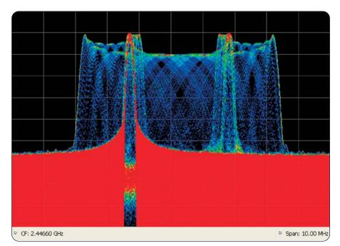
Revolutionary DPX<sup>™</sup> spectrum display reveals transient signal behavior that helps you discover instability, glitches and interference. Here, an infrequently occurring transient is seen in detail. The frequency of occurrence is color-graded, indicating the infrequent transient event in blue and the noise background in red.
