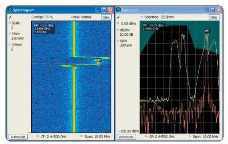
Trigger and Capture: The frequency mask trigger monitors for changes in the frequency domain and captures any violations into memory. The spectrogram display (left panel) shows frequency and amplitude changing over time. By selecting the point in time in the spectrogram where the spectrum violation triggered the FMT, the frequency domain view (right panel) automatically updates to show the detailed spectrum view at that precise moment in time.
